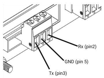
N.B Wire colours may vary between 3rd party cables/adapters (Pin numbers refer to a standard DB9 connector)
